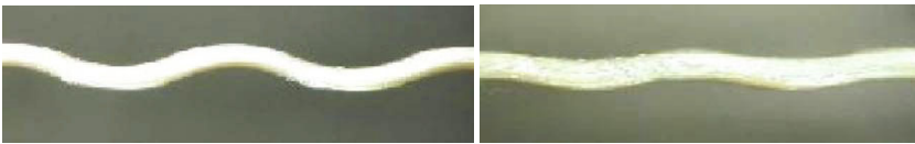
Figure 5.4. Crimp in warp (left) and weft (right) yarns from Twaron™ CT716 fabric (Tan et al, 2005).
