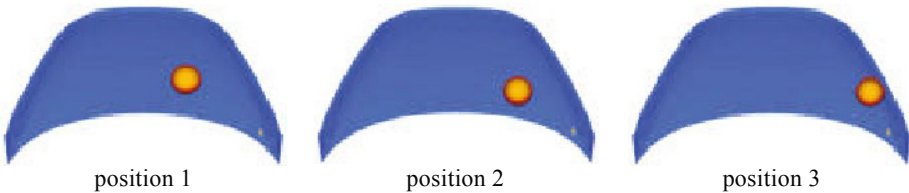
Figure 6.15 - The three headform-hood impact positions taken into account.
