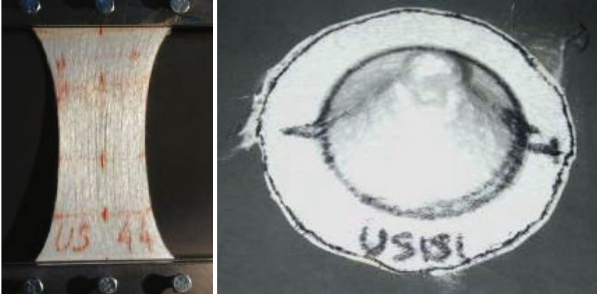
Figure 5.7. Left: Snapshot of an originally square specimen of Fraglight during a tensile test. Right: A close view of a Fraglight specimen tested with a drop weight tower. (Chocrón et al. 2008).
