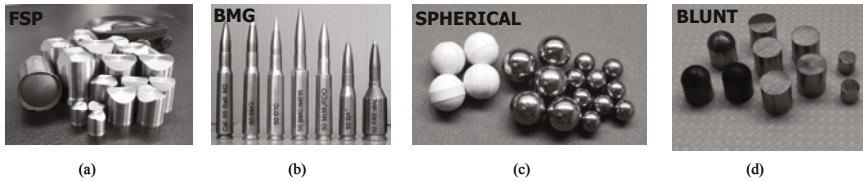
Figure 27. Typical projectiles used in ballistic impact; (a) Fragment simulating projectile; (b) Browning machine gun ammunition; (c) spherical hard ceramic or metal balls, and (d) blunt, hemispherical and flat head. Typical diameter range from 0.22 caliber to 0.50 caliber.
