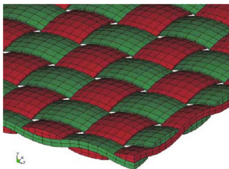
Figure 7.12. Finite element model for a plain-weave fabric structure (Duan et al. 2005).
